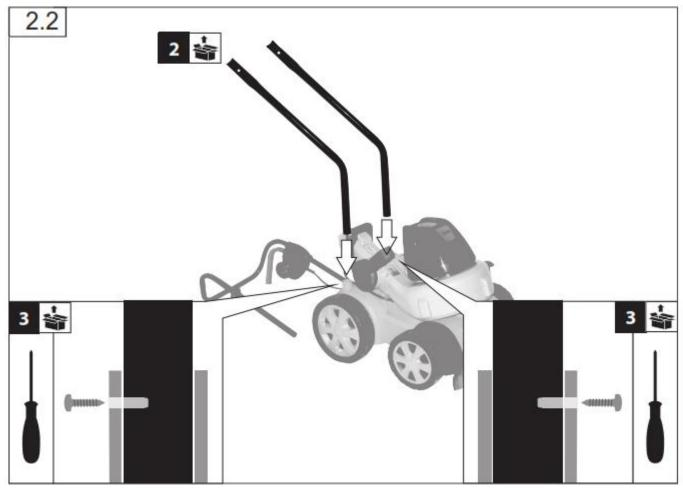
2.3.Connect and lock the upper bar and lower bar with square neck bolts & with two-Angle button(4).
